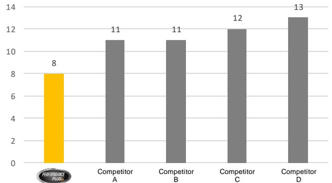
Performance Plus® uses KLEEN+ base oil to provide exceptional volatility performance resulting in less oil top off, less light end engine deposits, and excellent cold and high temperature viscosity performance v. conventional formulations.
