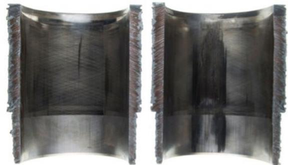
The image on the right shows damage from wear, and the image on the left show the protection provided by Performance Plus. The greatest amount of wear occurs at low temperature start-up, Performance Plus® is formulated to protect critical transmission components in these conditions to greatly extend the life of your transmission.
