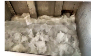
Powerful underwater jets enhance the platform-agitation cleaning process.
