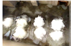
Powerful underwater jets enhance the platform-agitation cleaning process.
